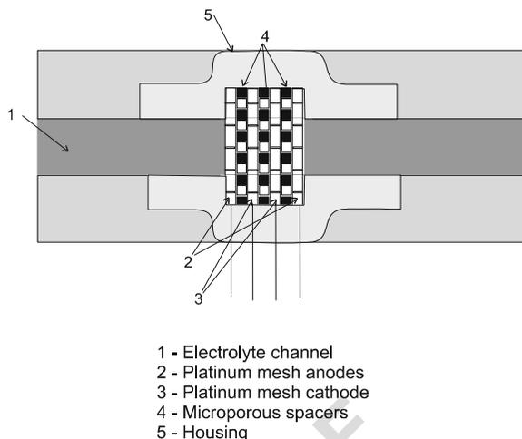
**Fig. 1** Electrochemical transducer
