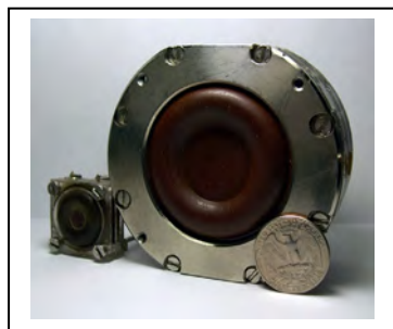
Figure 1. Progression of miniature sensor elements of a seismometer
